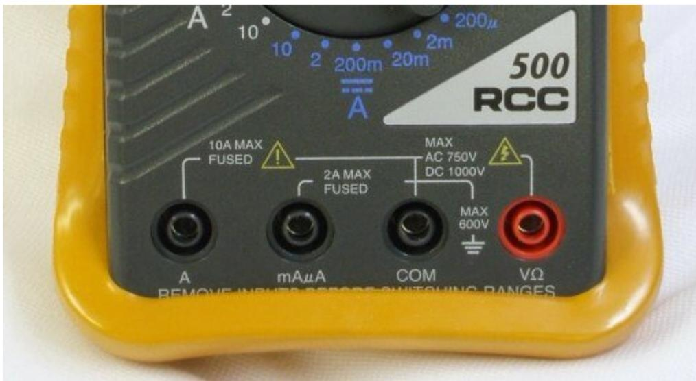
**The Common (negative) lead ALWAYS fits into the "COM" socket. The red lead fits into the red socket for Voltage and Resistance. Place the red lead (red banana plug) into "A" (for HIGH CURRENT "Amps") or mA,uA for LOW CURRENT.**
